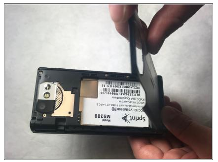
• Pull up on the back cover and lift the top to separate it from the phone.
