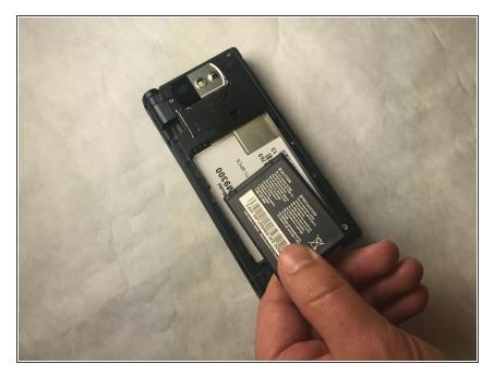
Pull the battery out of the device with a thin object such as your nail or credit card.
