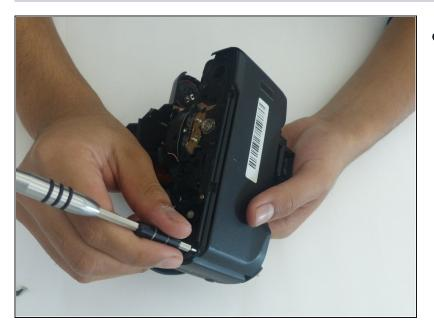
Once the front, top, and bottom covers have all been removed, it's time to remove the back latch! Using a paperclip or something similar (anything that's very skinny), push on the end of the skinny, silver, metal rod that vertically travels through the camera. Do this until enough of the rod pops out on the other side for the next step.
