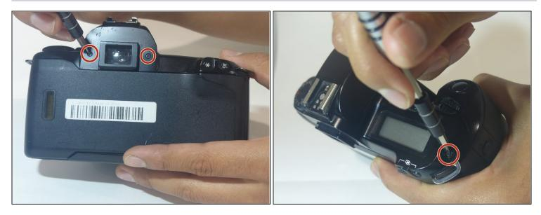
• Using a PH000 screwdriver bit, remove the three black screws shown in the two pictures that are all 4 mm in length and 1 mm in diameter.
