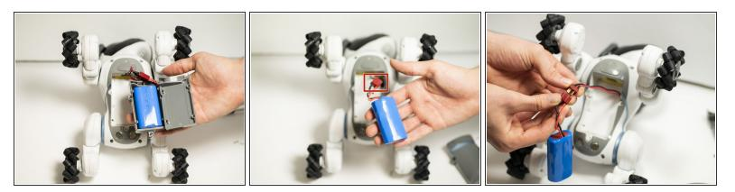
Once the battery is removed from body, the battery should be connected by a red and black wire. There is a red rectangular connector that easily pulls apart. Pull apart the red rectangular connector.
