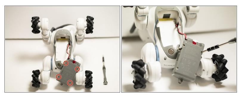
Once the top face of the battery is off, you will see a small rectangular box that the batteries are inside. There are 4 Phillips head screws in the box. Remove all screws with a Phillips head screwdriver.
