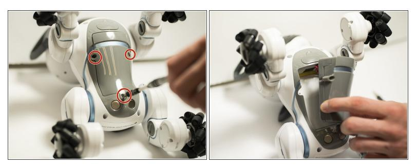
There are three small hex screws connecting the battery to CHiP. Remove all screws with a hex screwdriver and remove battery casing.
