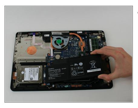
Lift the battery and remove it from the laptop.
