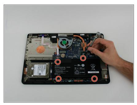
Unscrew the four 6mm screws with the Phillips #0 screwdriver.
