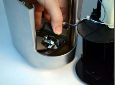
Remove the time/on switch by pulling upwards.
