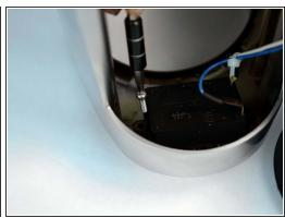
Remove two 11.59mm T10 screws.
