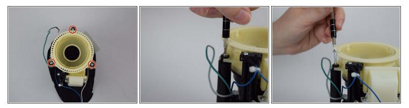
• Remove the three 19.61 mm T10 screws surrounding the white plastic burr housing.
