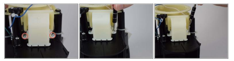
• Remove the two 13.60 mm T10 screws holding the bean chute to the base.
