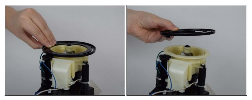
• Grab the edge of the plastic black ring that sits on top of the device and gently pull up to release.
