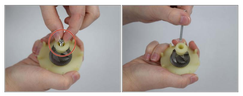
• Remove the loosened screw by pulling it upwards.
