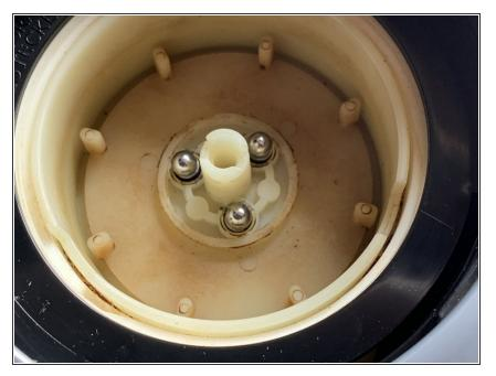
This is the correct position of bearings and springs when the screw and bottom burr are removed.
