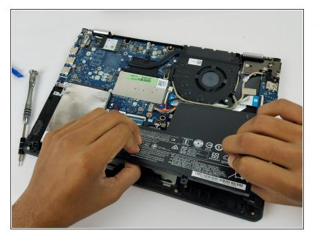
• Lift the battery up and out of the laptop.
