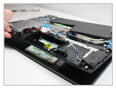
• Lift the base of the laptop from the screen and gently push the touchpad to remove.
