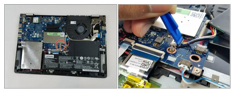
Disconnect the battery connector by using a plastic pry tool or your fingers to push the cable right towards the battery.
