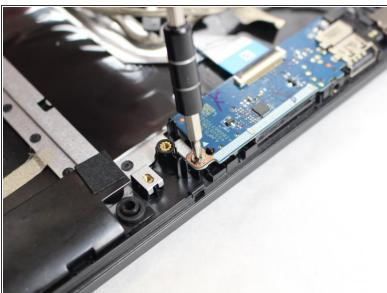
Remove the 4mm screw with a JIS #0 screwdriver.
