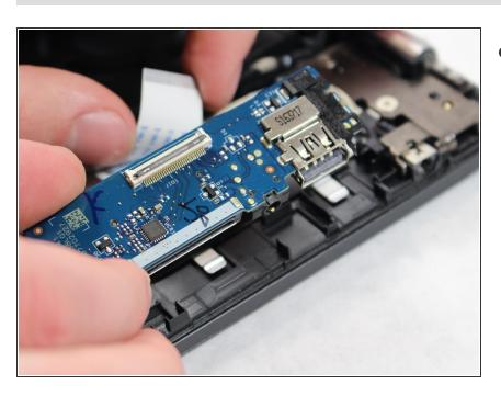
Remove the existing USB hub and replace it with the new hub.
