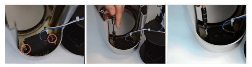
Remove two 11.59mm T10 screws.
