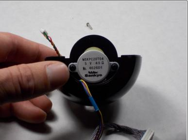
Pry apart the camera housing with your fingers to reveal the second motor.
