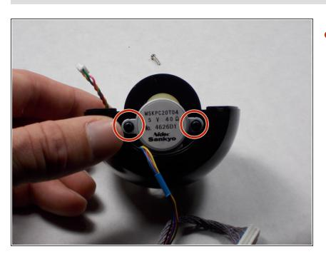
Unscrew the two 6mm screws holding the motor in place with a #1 Phillips screwdriver.
