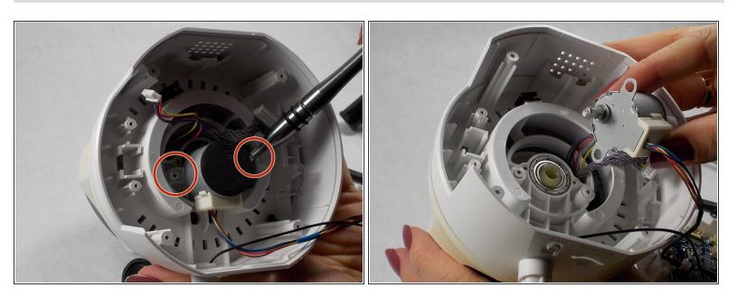
Use a #1 Phillips screwdriver to remove the two 7mm screws holding the motor in place.
