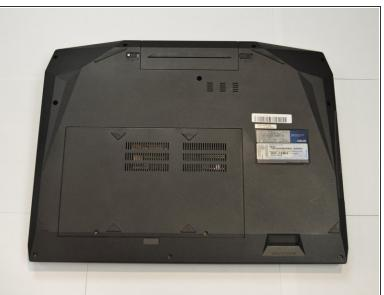
Flip the computer over, so that the bottom is facing up.
