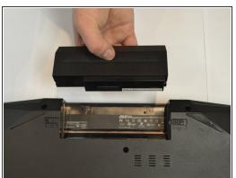
Use one hand to hold the non-locking tab in place, and use your other hand to pull the battery away from the computer.
