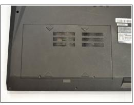
With the bottom of the computer facing up, remove the two 7.1 mm screws using a Phillips #00 screwdriver.
