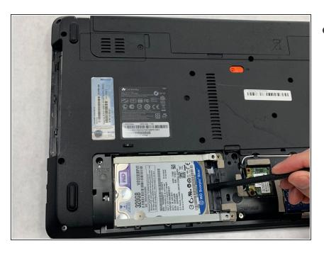
Push spudger to the left until hard drive is moved from its original position.
