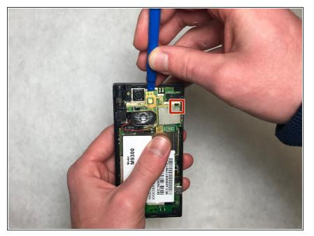
Wedge a plastic opening tool under the motherboard directly above the flash. Additionally, use a plastic opening tool to unhook corner labeled in a red square.
