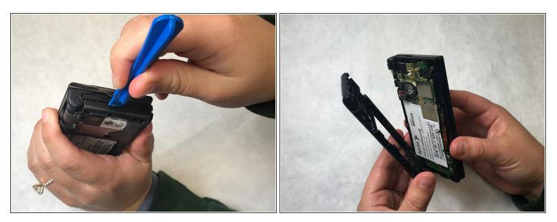
• Wedge a plastic opening tool under the black outer casing of the phone. Push the plastic opening tool down and outward while rotating the phone to pry the black outer casing off.
