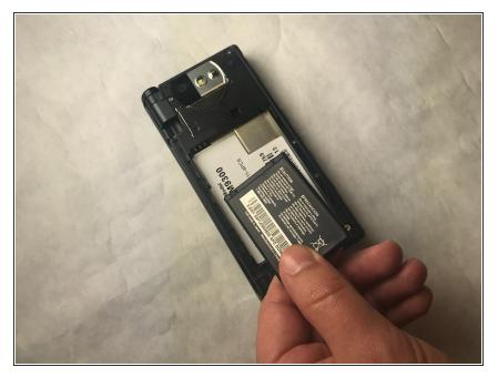
• Pull the battery out of the device with a thin object such as your nail or credit card.
