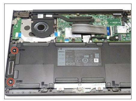
• Remove the four 2mm screws on the sides of the battery.
