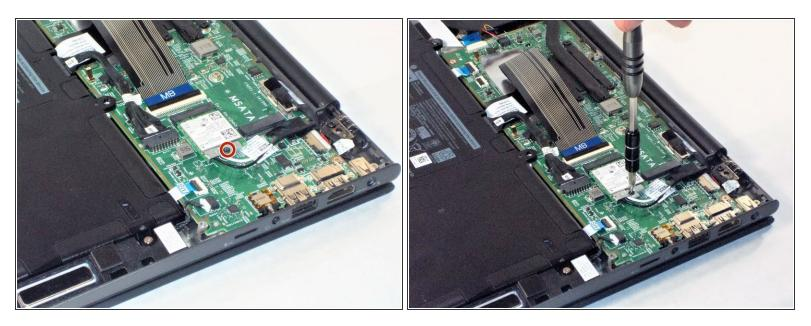
• Use #1 Phillips screwdriver to remove the 1mm screw in the network card.
