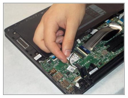
• Disconnect the network card from motherboard socket.
