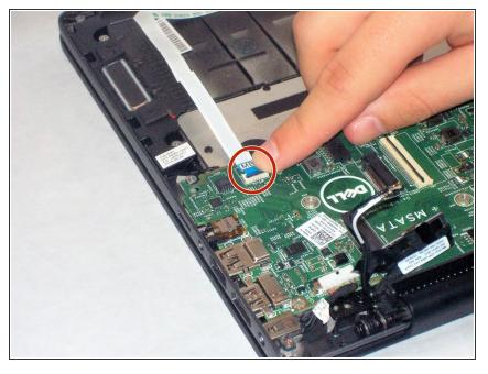
• Release cable for the LED charging indicator by pulling up on connector.
