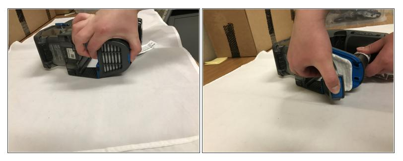
Press the blue lever located at the bottom of the handle and pull the plastic cover away from the main vacuum.
