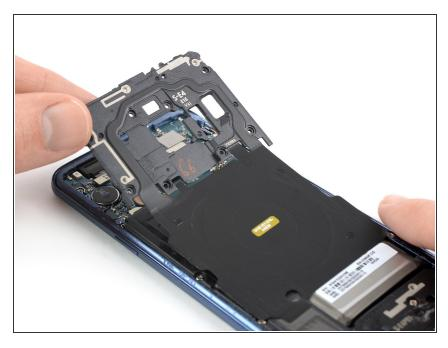
Remove the plastic cover containing the NFC antenna and charging coil. **If possible**, turn on your phone and **test your repair** before installing new adhesive and resealing the phone.
