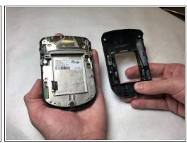
Grab the back housing from the bottom and lift the housing away from you.
