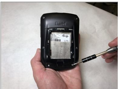
Remove the two 5 mm Torx T6 screws.
