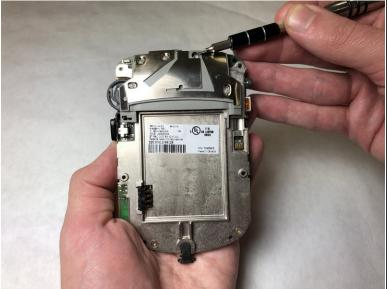
Remove the single 5 mm Torx T6 screw.
