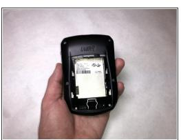
Remove the battery from the compartment.
