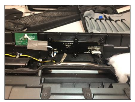
Underneath the cover, there is a black panel screwed onto the cover with two sets of wires plugged into it.
