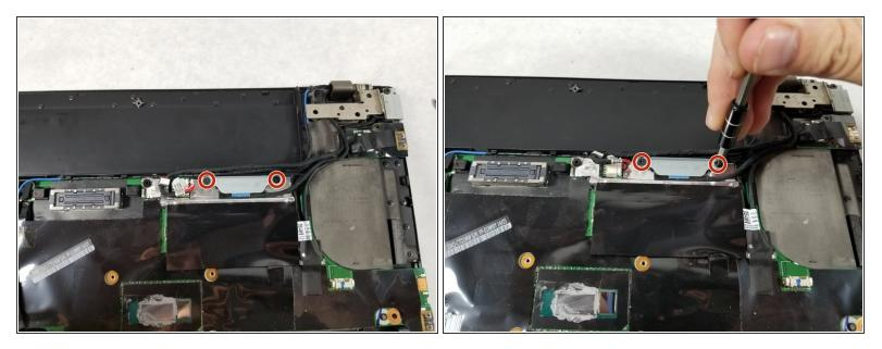
Use the Phillips #1 screwdriver to remove the two screws securing the metal plate to expose the wire connection.
