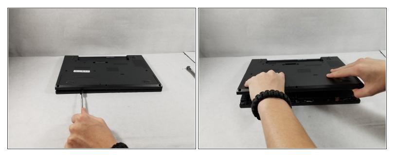
• Using the metal spudger, wedge it in the seam where the backplate meets the front plate and run the tool along the seam to separate the backplate.
