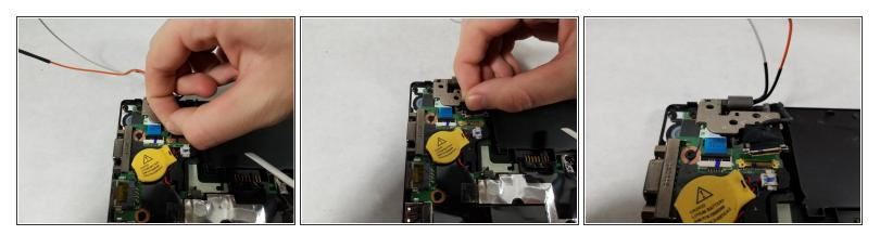
• Grab hold of the ribbon cable and pull it out of it's connection housing.
