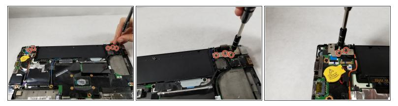
• Use the Phillips #1 screwdriver to remove the five screws securing the display mounts.
