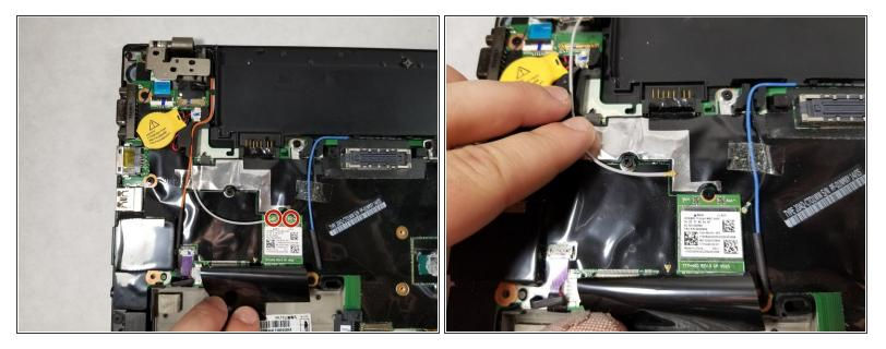
Disconnect the white and blue wires connected to the mounted circuit by grabbing them close to the connection and pulling upward.
