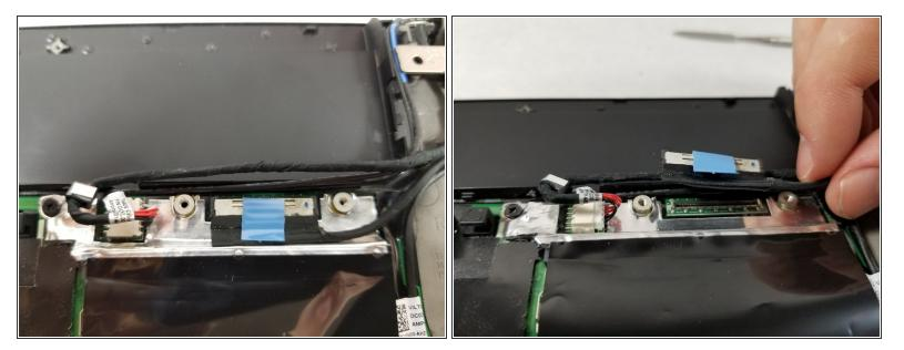
• Disconnect the wire by pulling it upward from the motherboard.
