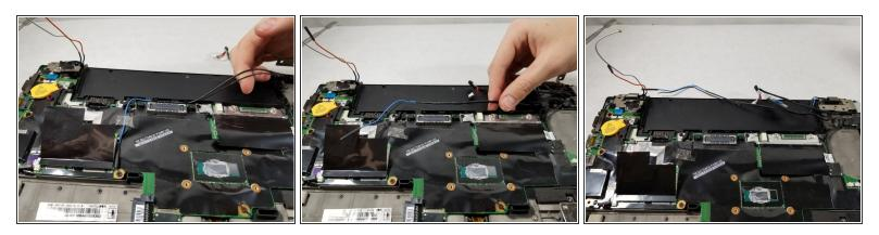
Unclip the 5 wires connected to the display assembly from the motherboard and move them out of the way.
