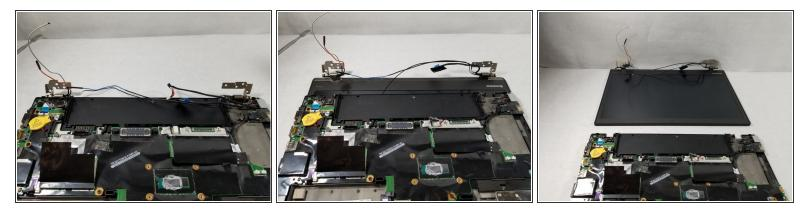
Now that the display assembly is disconnected from the main body, lift both of the mounting brackets and remove the display assembly from the main body.
