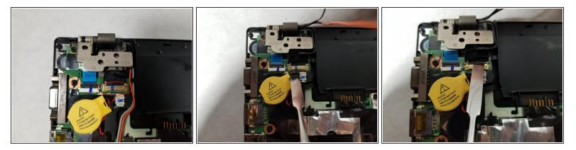
• Use the metal spudger to pry up the lever securing the ribbon cable in it's connection housing.
