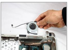
Once the screws have been taken out gently lift up the fan and remove it from the device.
