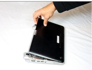
Gently lift the back panel of the laptop from where the battery was located.
