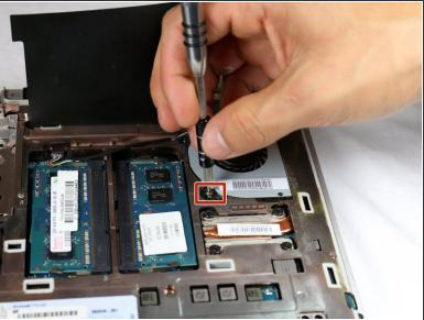
Remove the three screws with a #00 Phillips screwdriver.
