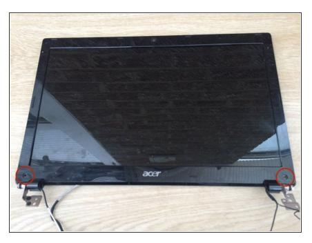
Open the laptop lid as far as it will go. Using a small craft knife or similar, remove the two black adhesive screw covers on either
