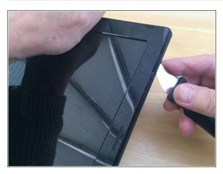
Separate the bezel around the screen by using a jimmy or similar tool to release the clips holding it in place. Work around both sides and the top. Finally, turn the laptop on its side in order to work along the bottom. You should now be able to lift off the bezel.
