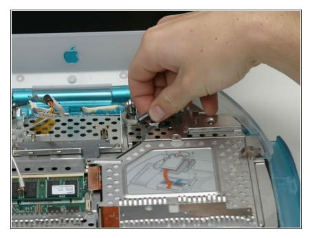
• Disconnect the backlight cable from the logic board and deroute it.
