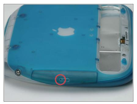
• Use a straightened paperclip to manually eject the CD-ROM tray.
