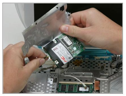
• Lift the modem partially out and disconnect the cable on the left side.
