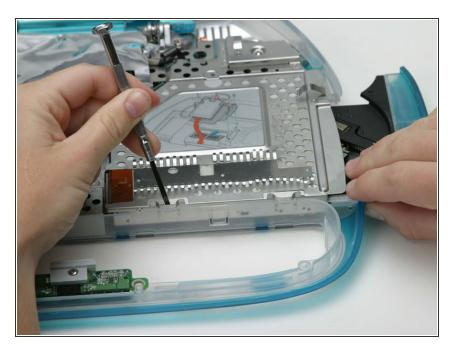
Lift up on the optical drive while sequentially pushing the small plastic tabs one after another toward
