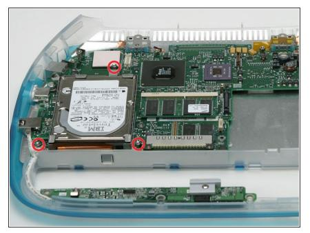
Remove the three 5 mm standoffs securing the hard drive to the logic board.
