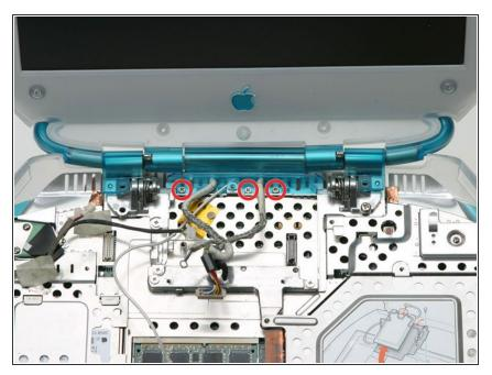
• Remove the three small Phillips screws from the clutch cover.
