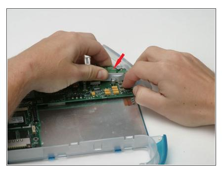
Push down firmly on the logic board and pull the DC-In board up from its connectors and then to the left.
