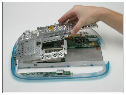
• Lift the right side of the EMI shield up and pull it out of the computer.
