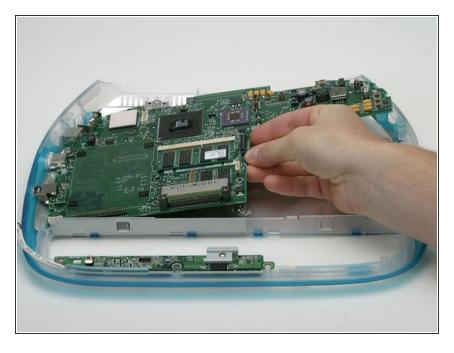
Grasp the logic board to the left of where the optical drive used to be and pull it up from the lower case.
