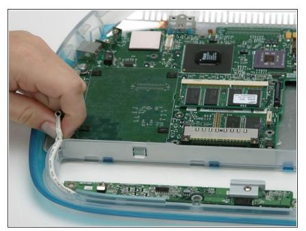
• Disconnect the charger board cable from the logic board.
