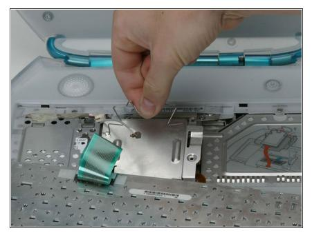
• Grasp the wire metal bracket on top of the RAM shield and pull upward to remove the shield.
