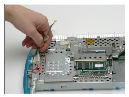
• Deroute the speaker cable from the metal framework and disconnect it from the logic board.
