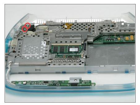
• Remove the two small Phillips screws from the RJ-11 board.
