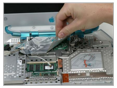
Peel the modem shield away from the metal framework below, working from the right front and moving to the left.
