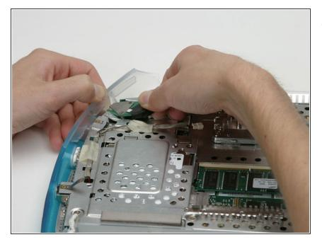
Push out the lower case rim and pull the RJ-11 board out of the computer.
