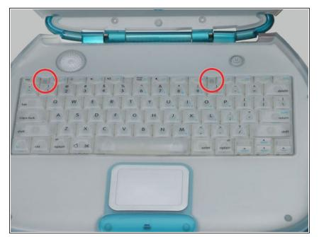
Pull the keyboard release tabs toward you and lift up on the keyboard until it pops free. Note that the keyboard ribbon is still attached to the logic board, so you cannot completely remove the keyboard yet.
