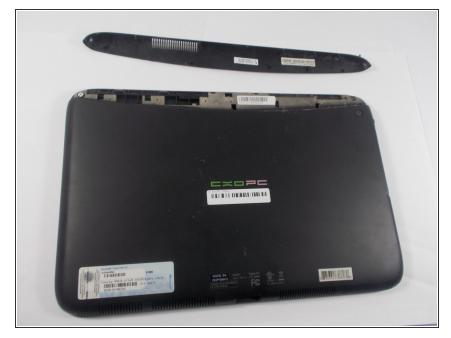
Turn the PC on its back with the screen facing down and pull on the piece of plastic shown in the image.
