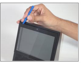
Use the plastic opening tool to gently lift the plastic protector from screen.
