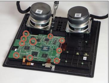
Unscrew the ten 1mm T5 Torx screws holding the motherboard in place.
