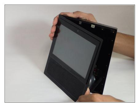
After the screws are removed, grip the front panel and remove, using a plastic opening tool if necessary.
