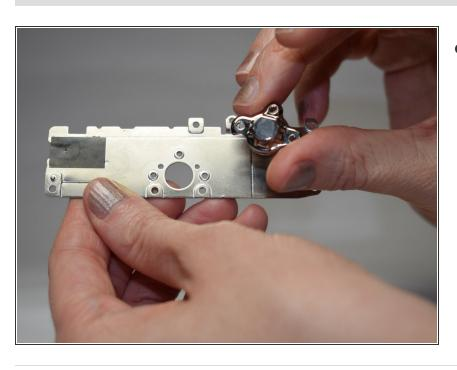
Remove the tripod mount from the metal plate.
