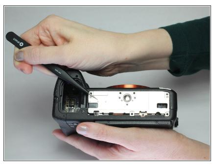
Remove metal plate. Sometimes this plate can become stuck and hard to remove. Use tweezers to separate the plate from the bottom of the camera.
