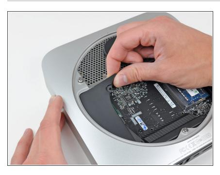
Lift the cowling from the end nearest the antenna plate.
