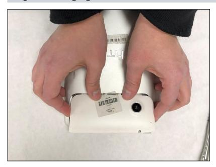
Remove the white portion of the top cover as shown. Push down on it to slide it off using just your fingers. Be careful not to break the clips holding it in place with removing it.
