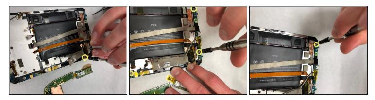
• Remove the motherboard. Note that the flex screen will not be removed with it and will remain attached to the tablet frame.
