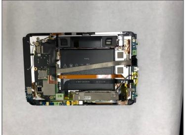
• Remove the plastic top cover of the motherboard.
