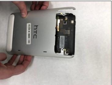
• Remove full frame on the back. A tip is to tape the volume button to the frame before removing it, as the volume button will fall out.
