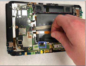
• Release the flex-screen touch cable. It is held in place with clips. Use the safe open pry tool to unclip it. Note that it will still be connected to the base and the motherboard.
