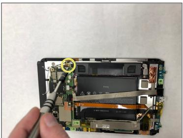
• Remove four T5 Torx screws.
