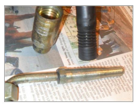
To remove each fitting, secure the outer shell in a vise or such. Use an open-ended wrench or flare wrench (better), to unscrew the mandrel tube from the ID of the hose. It is a normal right-hand thread. Once out, unscrew the hose from inside the shell. That is a left-hand thread, so turn as if you were tightening a bolt to unscrew.
