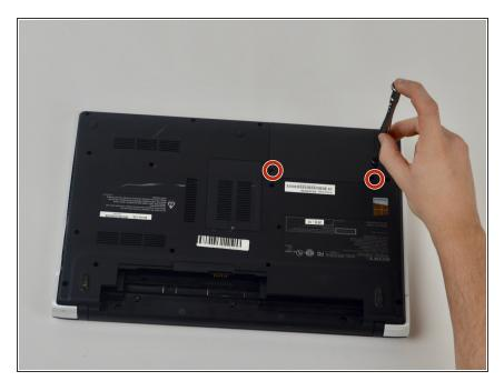
Remove 2 bottom screws in the top right on the HDD cover, with a size P000 screwdriver.
