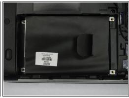
• Remove all four Phillips #00 screws that hold the hard drive in place.
