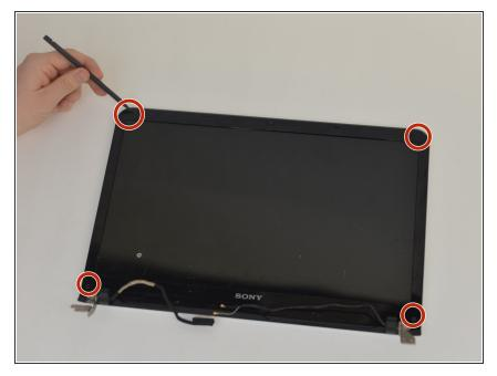
Remove the rubber nipples to expose the screws using the pointed side of the spudger.
