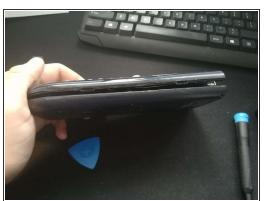
• Use a prying tool to get a pick into the side and then move it down until its open.
