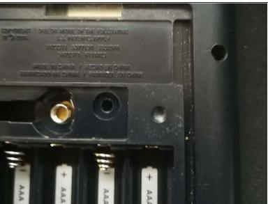
• remove the backup battery with either a screwdriver or the spudger.
