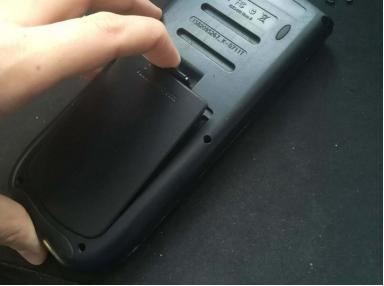
Press down on the latch, then remove the battery cover.
