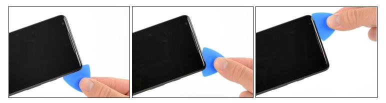
• Reinsert the flat edge of the pick at the top-right corner of the phone, and slide it around the corner and the top edge of the phone.
