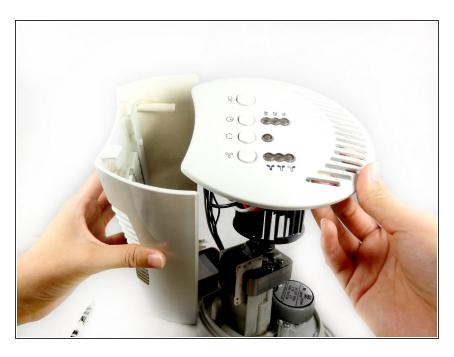
Remove the top cover containing the circuit board and the wires by pulling it away from the outer shell of the fan.
