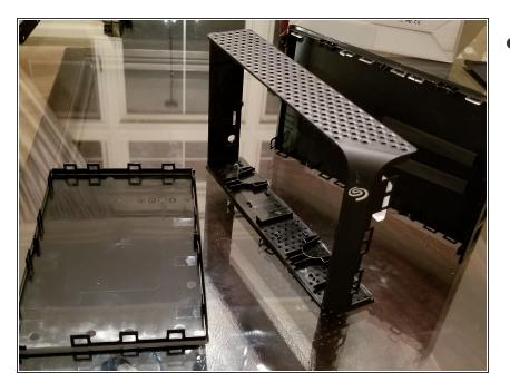
Above you will find a picture of the fully disassembled casing on the outside of the bay, (the board inside is not shown). The entire case is held togeter with snaps. These ones are particularly nasty and I found I could only prevent a few from breaking when opening the case even when using the gutar picks from the ifixit pro tech toolkit
