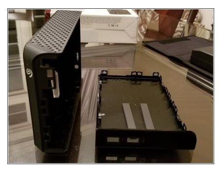
The rear casing plate is the only neccessary one to remove, above is a picture of the case when only the rear plate is removed.
