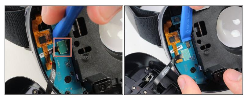
Use the iFixit opening tool to remove the pop connector holding the wire harness to the motherboard.
