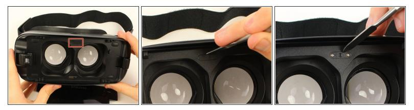
Use a metal spudger to remove the screw cover centered at the top.
