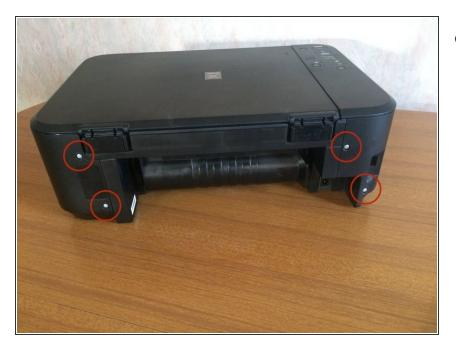
Remove 2 cross head screws from each side of the back of the printer.
