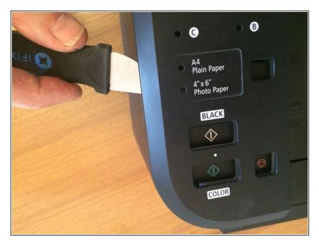
Using a jimmy (or similar tool), release the clips around the edge of the control panel cover, then lift off the cover.
