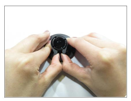
Hold two corners from the middle of bracket and stretch outward.
