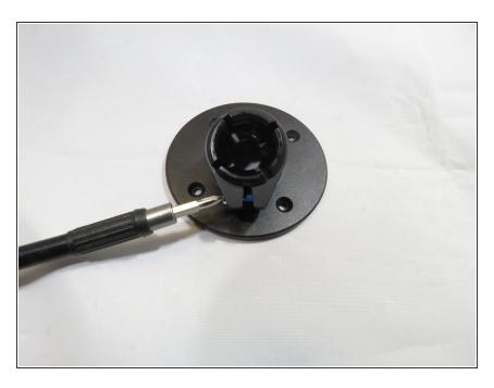
Use a Phillips #1 screwdriver to unscrew the single bracket screw.
