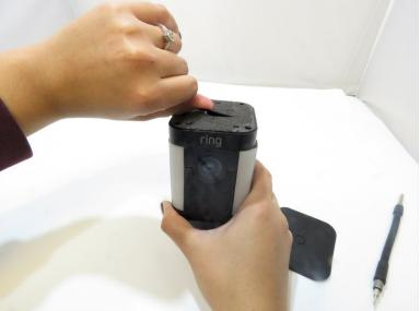
Remove the 7 PH00 screws around the four corners with PH00 of the lid.
