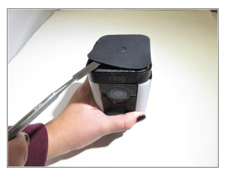
Remove the top plastic pad by peeling it off with a metal spudger.
