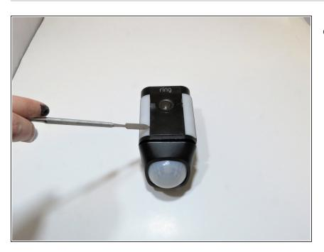
Use the metal spudger set to break the glue lining and the motion sensor will pop out.
