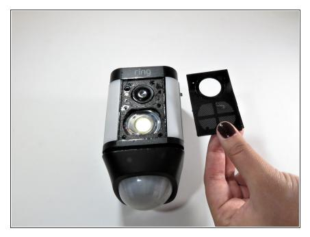
• Remove piece by pulling upward.
