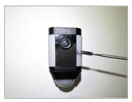
• Using metal spudger, place under sound mat and pull upward.
