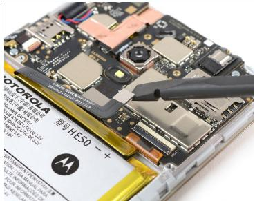
• Use the edge of a spudger to pry up and disconnect the battery flex cable from the motherboard.
