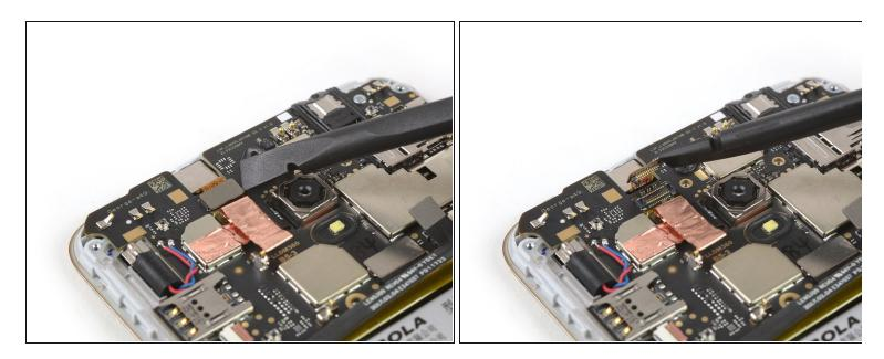
• Use the edge of a spudger to pry up and disconnect the front facing camera flex cable.
