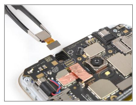
• Carefully remove the front facing camera with a pair of tweezers.
