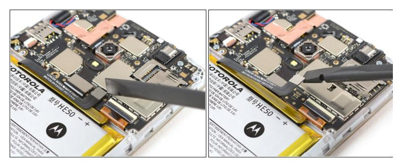
• Use the edge of a spudger to pry up and disconnect the battery flex cable from the motherboard.
