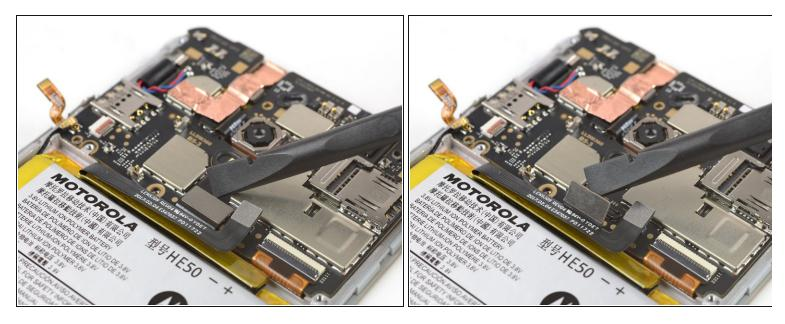
• Use the flat end of a spudger to pry up and disconnect the interconnect flex cable.
