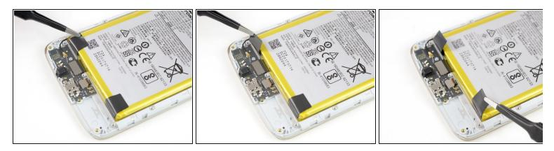
• Use a pair of tweezers to peel the ends of the two pull tabs off of the bottom edge of the battery.
