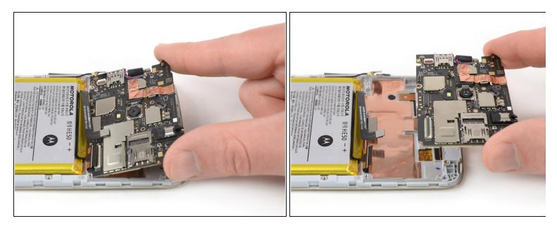
• Grasp the motherboard by the top corners and remove it by lifting up and pulling it carefully out of its recess.
