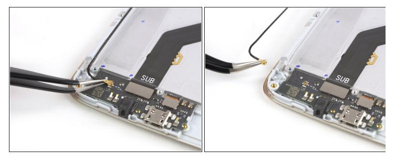
• Use a pair of tweezers to pry up and disconnect the antenna cable and remove it.
