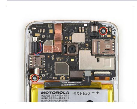
Remove the two 2.9 mm Phillips screws.
