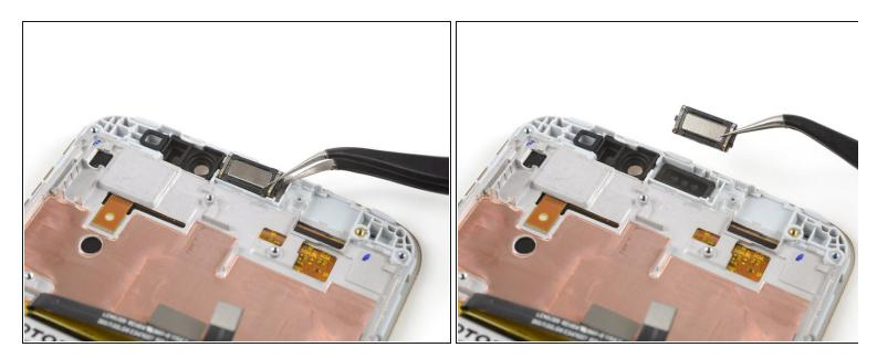
Multiply When removing the earpiece speaker with a pair of tweezers, take care to grab the whole unit. The earpiece speaker can easily break in two pieces if you only pull on its upper half.
