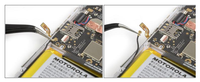
• Use a pair of tweezers to pry up and disconnect the antenna cable.
