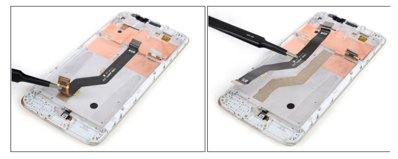
• Use a pair of tweezers to gently peel the interconnect flex cable from the frame and remove it.
