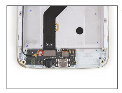
Remove the single 2.9 mm Phillips screw holding the charging board to the frame.
