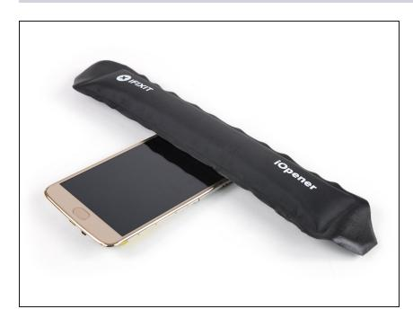
Apply a <u>heated iOpener</u> to the upper part of the phone for about 30 seconds to loosen the adhesive beneath the earpiece speaker.
