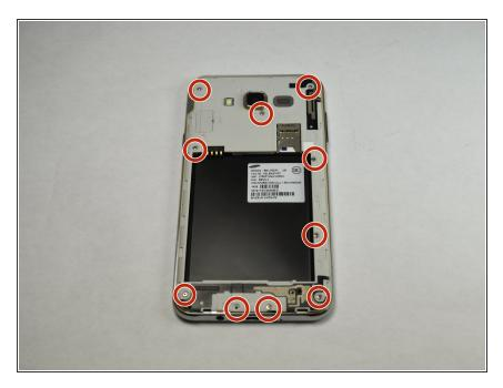
Using the Phillips #000 screwdriver, remove ten 4.2 mm screws.
