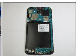
• Lift up the back of the device with the iFixit opening tool and disconnect it from the front.
