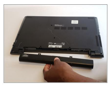
Pull the battery toward yourself until it is completely removed from the laptop. The battery should detach easily.
