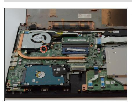
Use the Phillips #1 screwdriver to remove the screw securing the fan.
