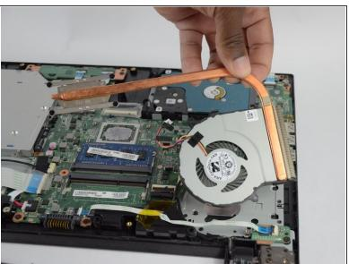
Pull the fan and heat sink away from the motherboard.
