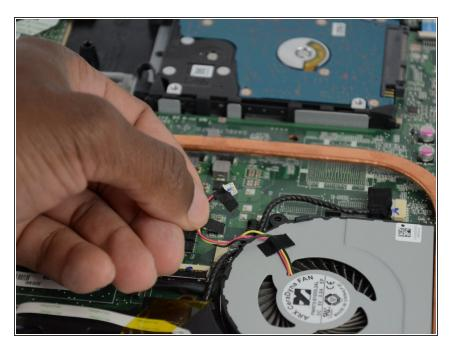
Disconnect the fan from the motherboard by removing the white holder with the red, yellow, and black wires.
