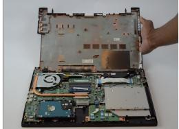
• Use the metal spudger to remove the bottom cover of the laptop.
