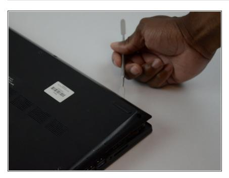
Run the metal spudger around the seam between the back cover and the rest of the laptop.
