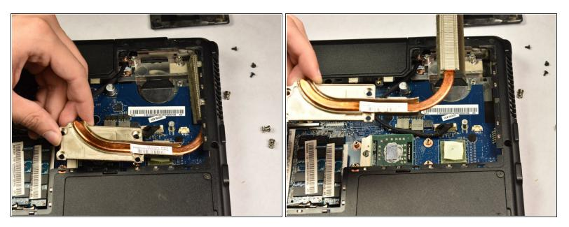
• Pull the heat sink assembly out of the laptop.
