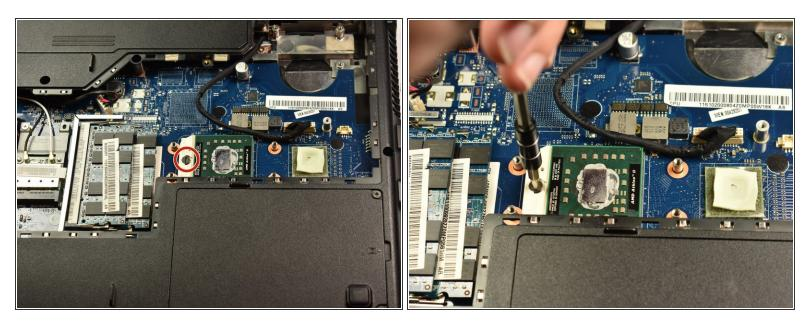
• Use a flat-head screwdriver on the hinge shown, and turn counter-clockwise to the unlock position
