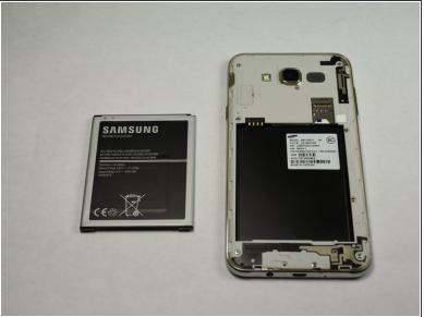
Pull out the battery by pulling on the bottom left slit under the battery.
