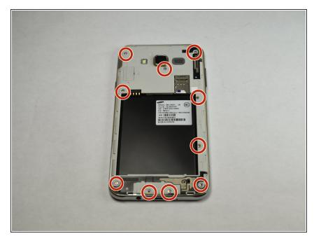
Using the Phillips #000 screwdriver, remove ten 4.2 mm screws.
